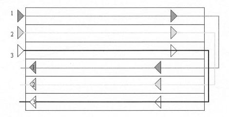
The *grid method* is basically the strip method performed in two directions. After searching in one direction, the searcher proceeds in a perpendicular direction. This technique allows for the same area to be searched twice. The method is efficient and thorough for large areas using any number of searchers. It is the most effective search method for almost every situation.
